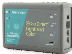
This light sensor measures light in the visible and ultraviolet electromagnetic spectra. An RGB color sensor detects relative contributions of primary colors in light. The Go Direct Light and Color Sensor directly connects wirelessly via Bluetooth or wired via USB to your platform. The sensor can be used for the study of visible light intensity, UV light intensity, and color investigations.
