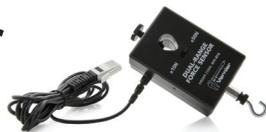
The Dual-Range Force Sensor is a general-purpose device for measuring pushing and pulling forces. It can be used as a replacement for a hand-held spring scale or mounted on a ring stand. It can also be mounted on a dynamics cart to study collisions. Forces as small as 0.01 N and as large as 50 N can be measured. The Dual-Range Force Sensor can be used for a variety of experiments, including
