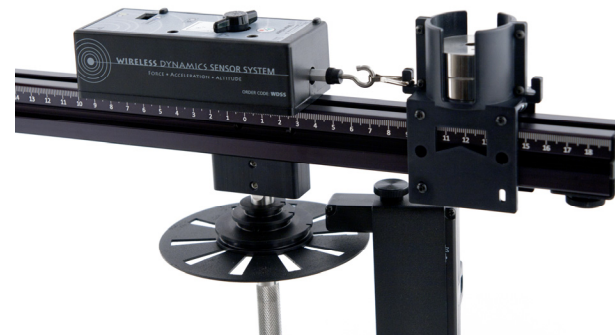
WDSS attached to beam and Sliding Carriage
