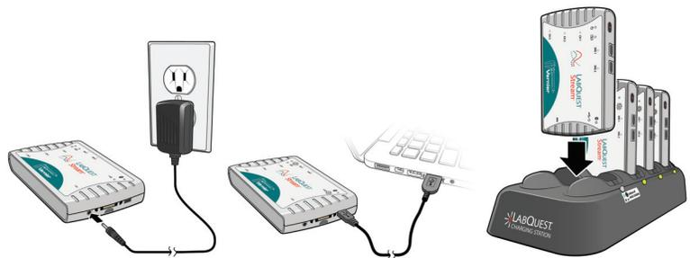
The Charging LED,
